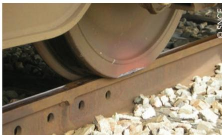
PLATS AUX ROUES SUITE AU BLOCAGE DES ROUES LORS D'UN FREINAGE
